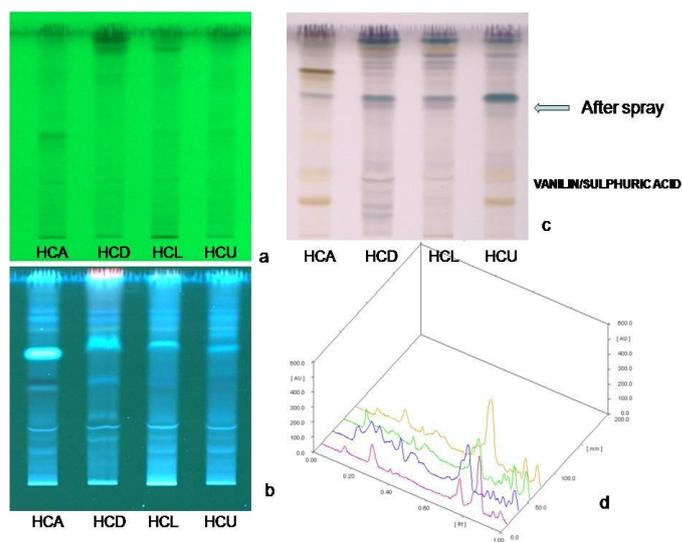
**Figure 6:** HPTLC fingerprint profile; HPTLC chromatogram visualized at 254 nm (a), 366 nm (b) and 600 nm (c) showing a TLC pattern of hydro methanolic (H) extracts. Pattern shown by 254 nm and 366 nm were recorded before derivatization while pattern shown by AS-600 nm was recorded at 600 nm after derivatization with vanillin sulfuric acid (d) HPTLC densitogram showing at 600 nm after derivatization.
