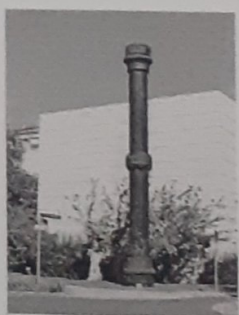
A historical (1921) high-pressure steel reactor for production of ammonia via Bosch-Haber process on the premises of the University Karlsruhe, Germany.
