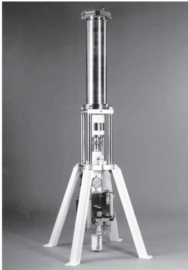
**Figure 6.18** Preparative HPLC column (15 cm in diameter) used in processing of proteins required for therapeutic or diagnostic purposes. Column manufactured by Prochrom, Nancy, France (photograph courtesy of Affinity Chromatography Ltd)
