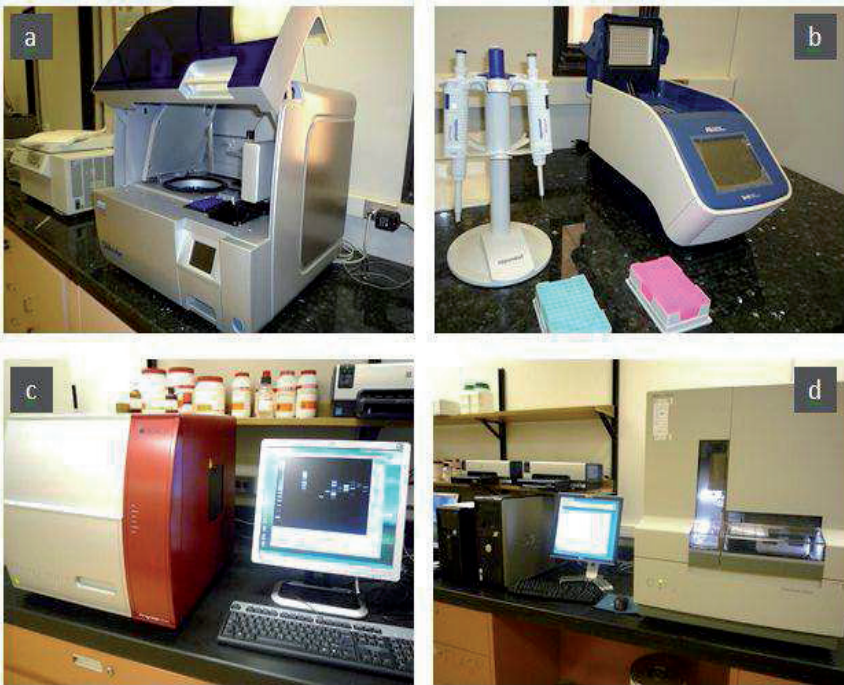
Fig. 1: Instrumentation setup for DNA sequencing (a) automated nucleic acids extraction system, (b) thermal cycler, (c) gel documentation and imaging system and (d) automated DNA sequencer.
